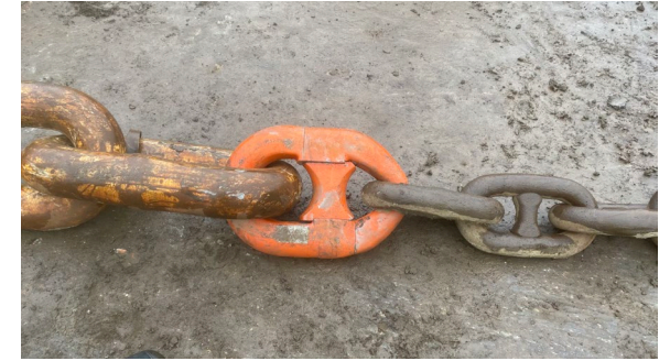
Trial fit connection between 159 to 84mm dia chain
