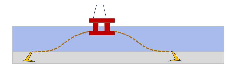
If there is no harm if a storm is coming and Rig operator can drop the anchors (disconnect) and sail on DP, the risk is minimal, and this should be reflected in the RP.
