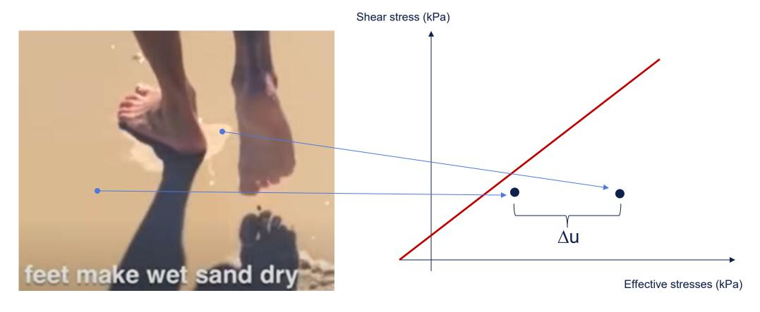
The soil around the foot gets an increased strength (due to suction)
